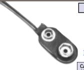
Cover Sizes:  $1.125 \times .530$ Contacts: Brass, Nickel Plate Wire: #26 AWG, 7/34 End Strip: .250 Long, Tinned
